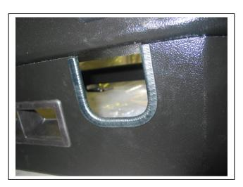
Figure 10: 3mm clip lock trim fitted
