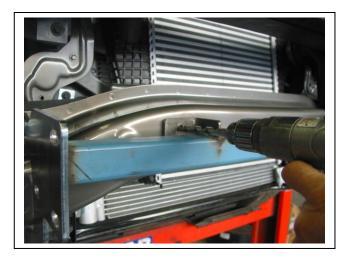
Figure 2: Drill holes to 10mm
