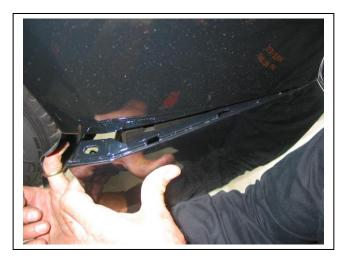
Figure 1: pull bumper rearward and out to release.
